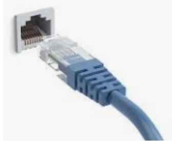
You can use this port to connect the DEVICE to an existing network (to a switch or to a router) or directly to the Ethernet port of a PC. All types of cables on the market are suitable, straight cables of type A or B and cross-over, because the DEVICES support the MDI/MDIX function for self-negotiation. Use UTP, STP or FTP network cable, with CAT5 or higher category.
