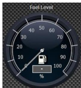
For example, in this case the fuel level is not detectable because it is not configured on the board.
