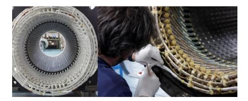
Each stator of the X-TYPE series of medium and high voltage is tested at all production stages, for example before and after the VPI (Vacuum Pressure Impregnation) cycle; in this way we guarantee the highest quality and reliability of the sold product.
