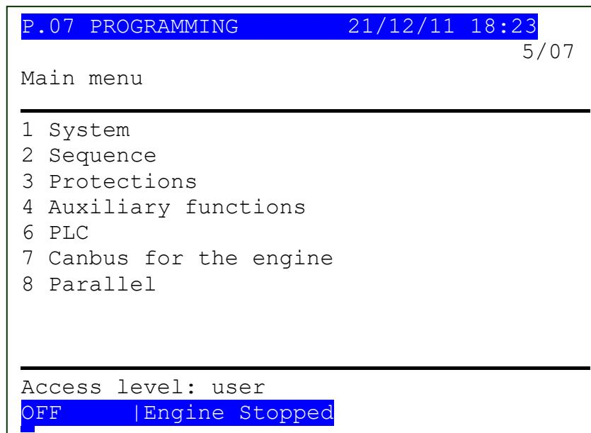
By pressing ENTER in 6-PLC, you activate the setpoint change procedure. On the DST4602 controller, 62 parameters are available starting from the index 1501.
