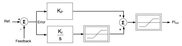
fig. 7: regulator diagram
