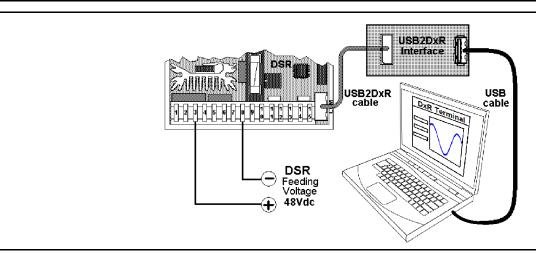
Fig. 11a: DSR 48Vdc power supply (please note that no other connections, other than the power source, are necessary) for the download of the alarms without risking to modify the content of the EEPROM because of the test.
