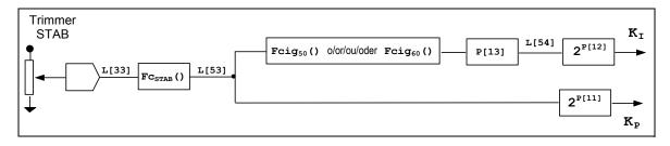
fig. 7a: drawing of the numeric elaboration of the proportional and integral gain by a DSR (standard) with the STAB trimmer enabled
