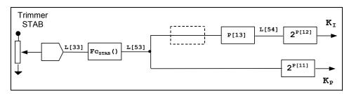
fig. 7b: drawing of the numeric elaboration of the proportional and integral gain by a DSR/A with the STAB trimmer enabled
