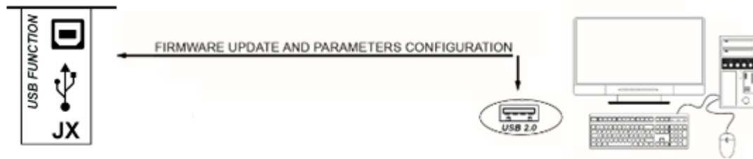
MP250 has a USB port with B-type connector for a temporary connection with a PC for the parameter's configuration or for the reading of history logs.
