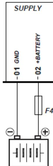
**⚠ ATTENTION!** To respect the safety rules, an isolation of the power supply from the public grid must be always guarantee and must be lower than the one of a safety transformer compliant with norm IEC61558-2-6 or equivalent.
