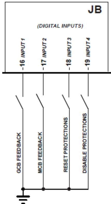
The controller has 4 digital inputs, which can be activated by connecting them to GND. When left unconnected, the terminals go to around 4.5 VDC (around 4.15 VDC for input T.16). Avoid situations where intermediate or undefined voltage levels can occur.
