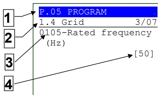
The second row always shows the name of the current menu (for example the "1.4 Grid" menu), followed by the numerical indication of the selected menu item and the number of items in the menu. The following rows of the display are all used to display a single parameter. In particular:
