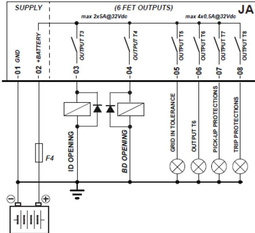
The device manages six digital outputs, fully configurable. When activated, they bring their terminals to the positive power supply voltage (terminal T.02); **make sure that any safety fuse on the power supply positive line has a capacity and response time suitable to power and protect both the outputs and the controller under any condition of use.**
