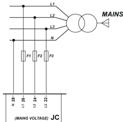
The terminals **T.22**, **T.24**, **T.26**, **T.28** allow the connection to the public grid, using protection fuses (suggested 1A).
