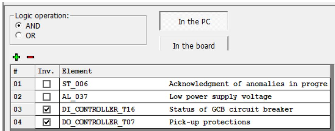
It is necessary to decide whether the list of conditions must be evaluated as AND (they must be all verified) or as OR (it is enough that at least one condition is verified). **It is not possible to have mixed logics AND/OR (it is possible using the virtual digital inputs, see afterwards).**
