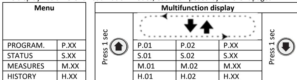
You can switch modes by holding down the **UP** or **DOWN** buttons for more than one second. Pressing them for less than a second, on the other hand, selects the pages within the current mode.
