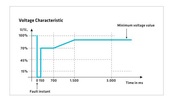
For type-1 generating unit, synchronous generator directly connected to the network (only through the generator transformer), the power station shall not disconnect even in the conditions shown in the pictures
