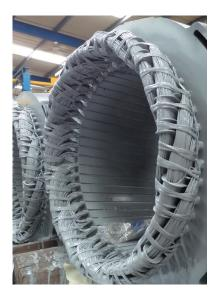
A Grid Code compliant generator must comply with both static and dynamic requirements of the appropriate Grid Code. In dynamic response the connection must remain while the Low Voltage Ride Through (LVRT) occurs, and survive the huge forces trying to change the concentric alignment of the stator.
