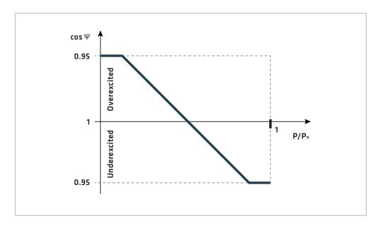
The reactive power of the generating plant must be adjustable. Any reactive power value resulting from the characteristic must automatically adapt within 10 seconds for inductive load and adjustable between 10 and 60 seconds for capacitive load
