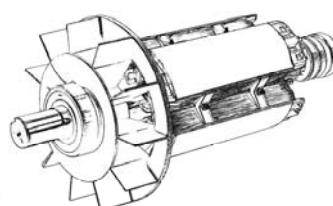
ATO/ATEB/AMEB-28 2 and 4 pole alternators are brush and brushless, self regulating and incorporate a rotating inductor with damper cage and a fixed stator with skewed slots. The stator windings have a shortened pitch to reduce the harmonic content of the output waveform. The alternators are made in compliance with the 2006/42, 2006/95, 2004/108 directives and their amendments, and the EN ISO 12100-1, 60204-1, EN 61000-6-2, EN 61000-6-3, EN 60034-1. regulations.
