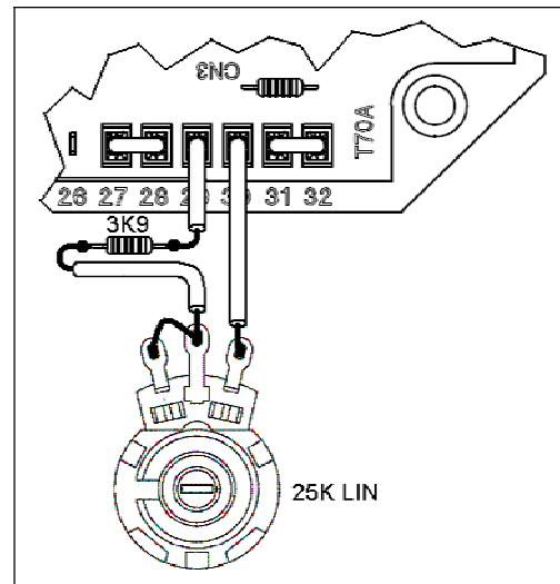
Figure 4b: 25K external potentiometer connec-
