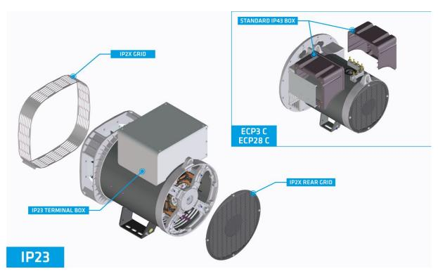
In this image you can see the standard configuration of our industrial generators. In some series the standard terminal box is in plastic, having a degree of protection of IP43 (the degree of protection of the complete generator will remain IP23).
