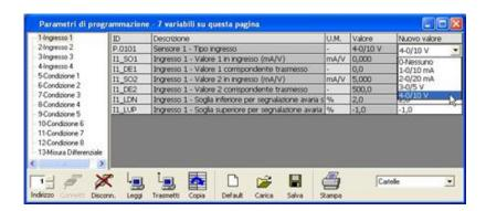
You can set the limits of acceptability of the signals from the sensors: these are the lower and upper thresholds for reporting sensor faults. Values are expressed as a percentage and refer to the current or voltage reading. E.g.: if we have a 4-20 mA signal, the input will be configured for 0-20 mA; we can set 20% as the lower threshold and 100% as the upper threshold so if the sensor signal is below 4 mA or above 20 mA a fault will be reported (sensor faulty or disconnected).
