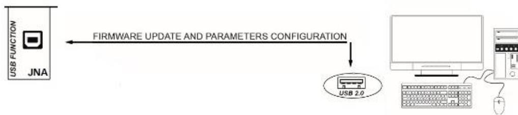
The USB protocol specifications don't allow its use in the permanent industrial field due to the limited length of the cable and of the elevated sensibility to electric disturbs also on PC side. For this reason, **the USB connection cable has to be inserted only when it is necessary to operate on the device and can be removed from the JNA connector when the operation has finished.**
