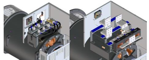
On C type family has been installed a new AVR panel. Terminal boards have been redesigned into a special L configuration, specifically to ease customer wiring; with this kind of terminal board it is possible to place a second terminal board in order to get 12 available terminals. Current transformers are available as an option on series ECO38 with single or dual output.
