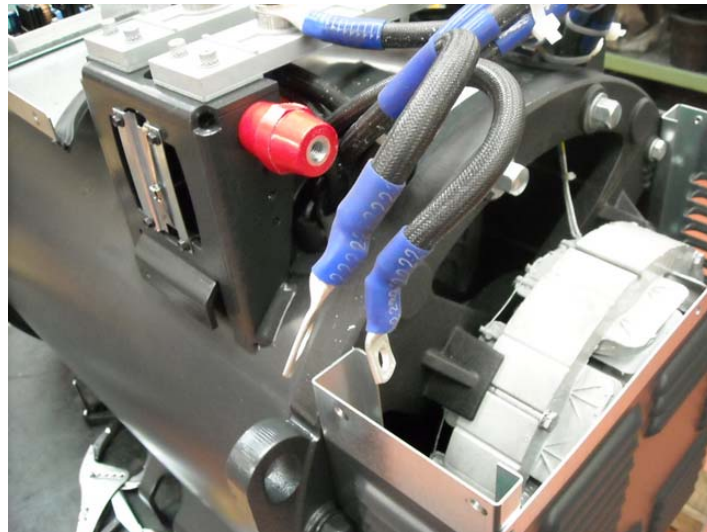
Fig.18 M16 n.2 power cable and M10 kit power cable terminals on the isolator
